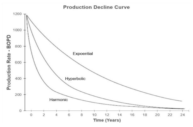
**Exponential:** An exponential decline is the most common type of decline seen in conventional oil and gas reservoirs and wells. The trend line has a constant slope signifying a steady decline in production over time.
